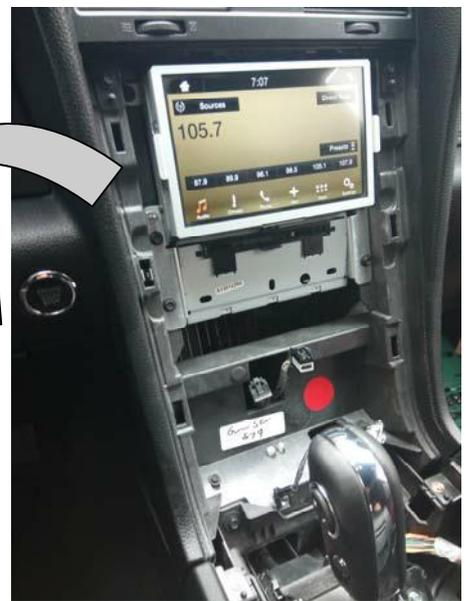
When the monitor is taken down from the car, the connectors behind are like this:
