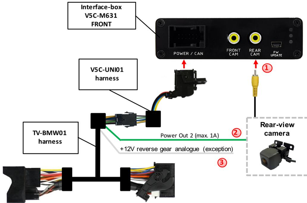
1 Connect the video RCA of the after-market rear-view camera to the female RCA connector "REAR CAM" of the interface box V5C-M631.
