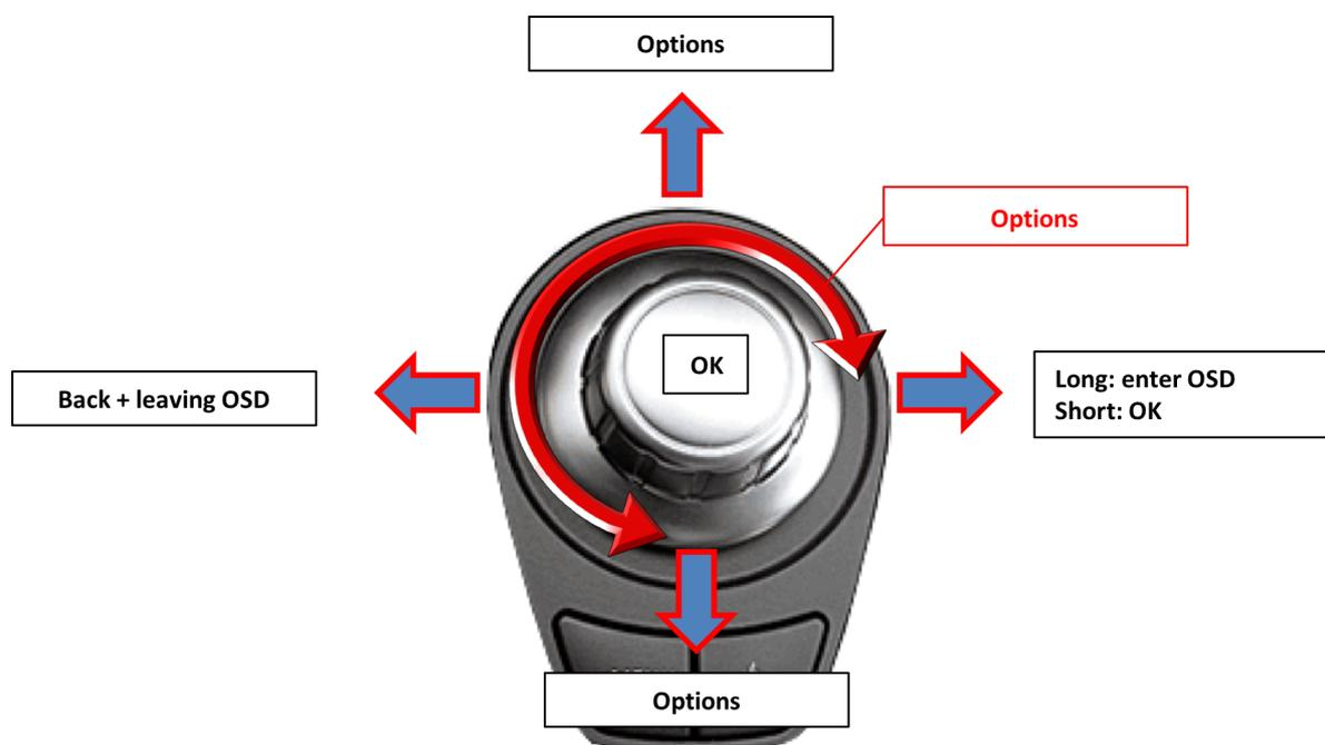
**Note:** If the interface is selected as active video source then the OSD menu is activated via iDrive button "OK" (press and hold) + "iDrive-right". In this OSD menu only image adjustments can be made.
