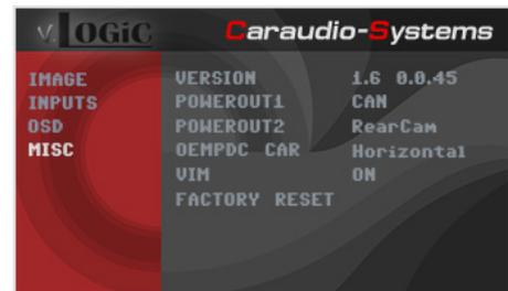
3 On some vehicles the reverse light signal doesn't exist on the CAN-bus. Connect the white wire of harness TV-BMW01 to reverse light signal (+12V of reverse light) if the system doesn't switch to the rear-view camera automatically after the described OSD-setup (see next chapter).
