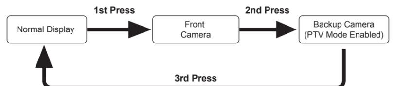
\* Selecting reverse gear will display the backup camera and override the front camera display (if currently selected). Shifting out of reverse gear will then return to the normal display screen regardless if the front camera was previously selected (default settings only).
