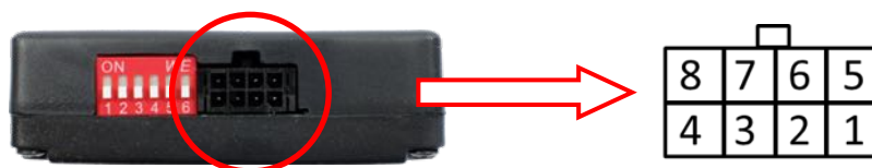
Pin-assignment male 8pin connector of TV-500
