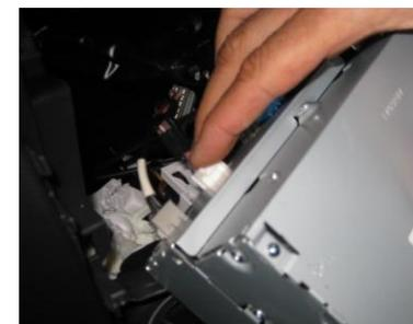
9. Refit the head unit by following the previous steps backwards. Connect the 12 way micro-fit (12 pin molex) to the Car side of the Dension SBK module – behind the glove box.
