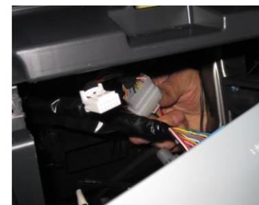
8. Connect the 12-pin connector on the car side harness to the CD changer connector on the back of the head unit.
