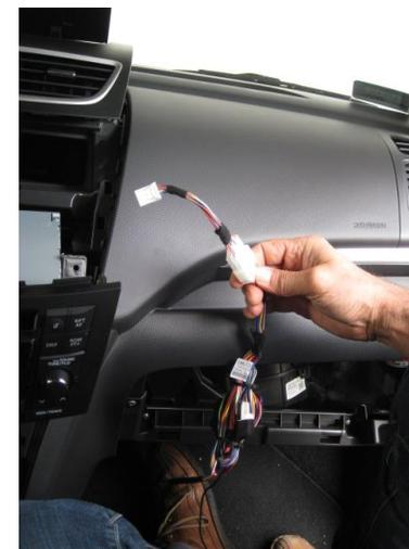
7. Run the car side harness through the glove box to the back of the head unit.
