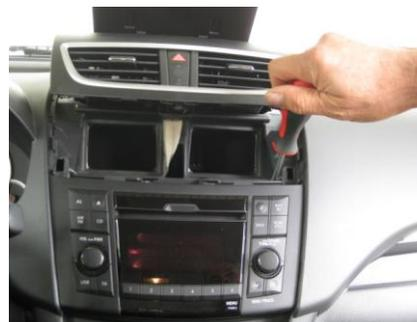
4. Remove the head unit by pulling it out horizontally.
