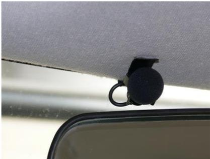
11. Run the microphone cable under the roof lining all the way up to the plastic cover on the 'A pillar'.
