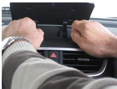
3. After lifting the air vent panel, remove the two PH screws above the head unit.
