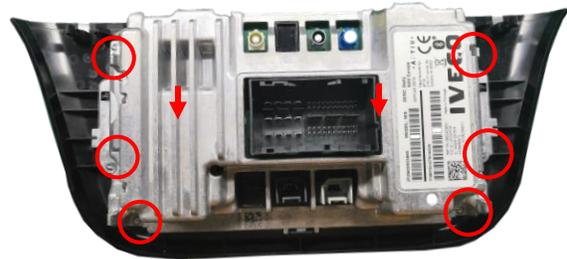
2、 Remove screws, then the rear can be opened.
