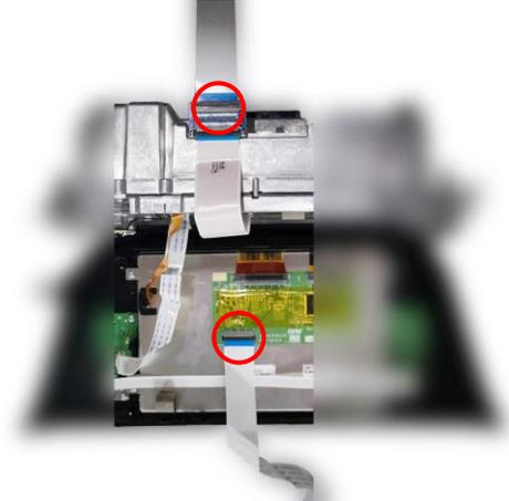
4、 Put the OEM ribbon to the external PCB and connect interface's 200mm ribbon connect to OE socket .
