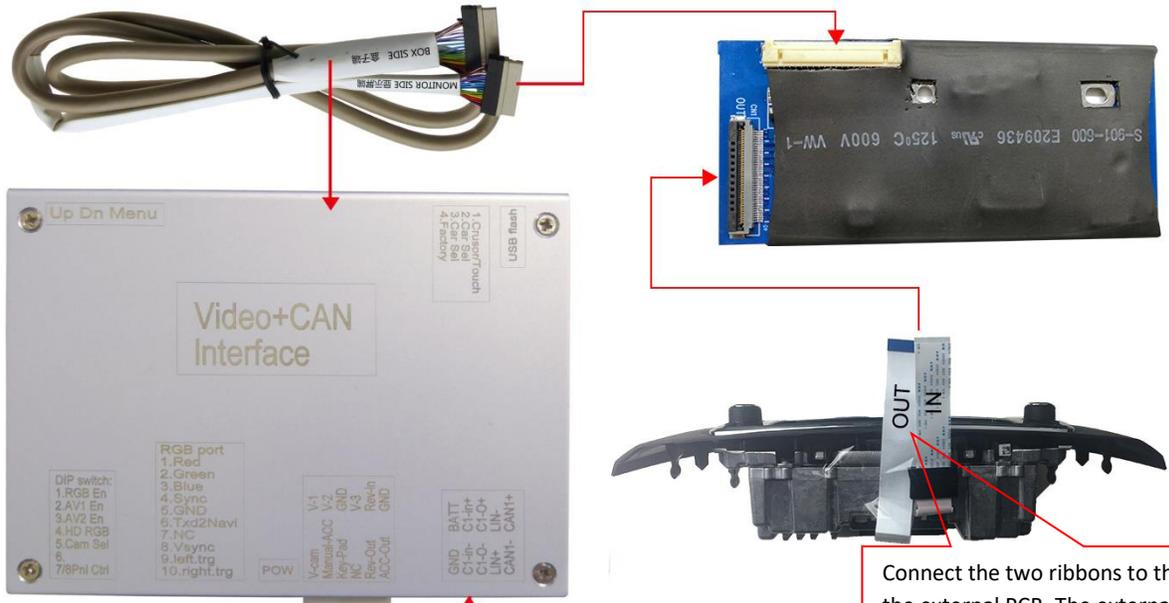
Connect the two ribbons to the two sockets on the external PCB. The external PCB sockets are signed OUT and IN. Connect the ribbon IN to the socket IN and ribbon OUT to socket OUT (the ribbon connected to the 40pin external PCB is IN). The PCB installation will show how to connect the ribbons and boards.
