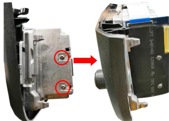
6、 Remove the screws and put our external PCB on the HU, then fix the external PCB by the screws as the above picture shows.
