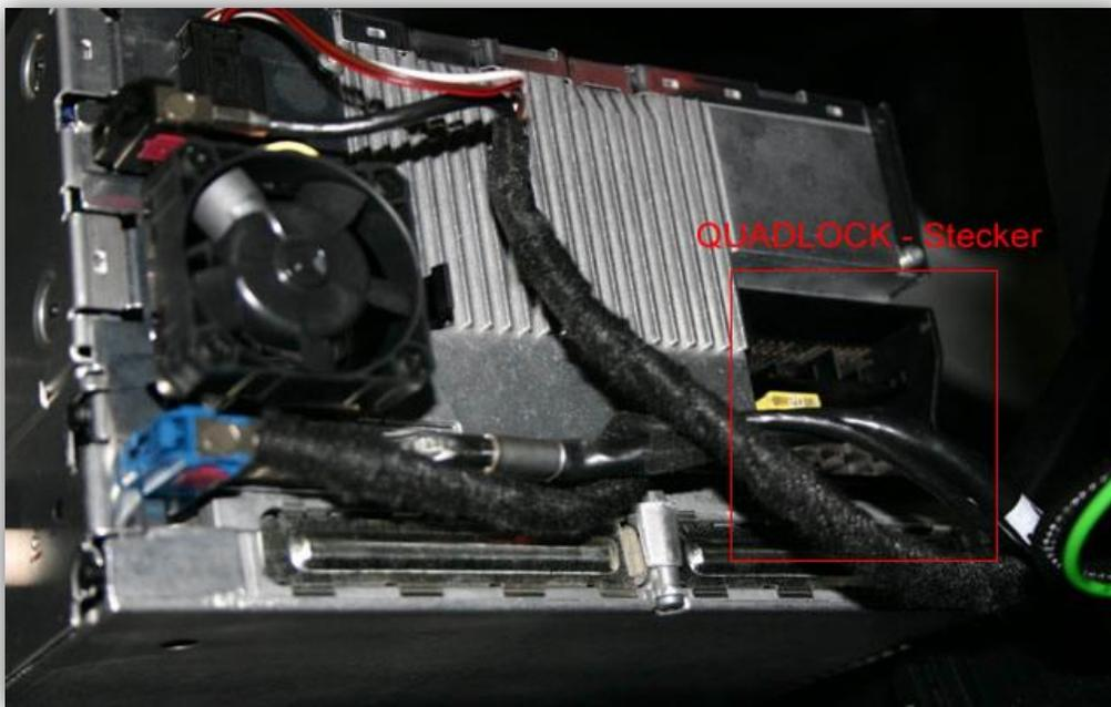
The Quadlock connector includes different chambers. If present, remove the white, black and the optical inserts, from the vehicle harness' Quadlock connector. Plug the vehicle harness' Quadlock connector into the male Quadlock connector of the CAN interface harness TV-BMW01
