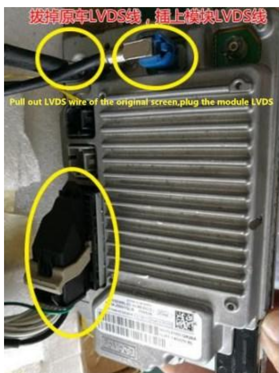
12.Plug the attaching plug of the original car screen,plug the module LVDS wire.
