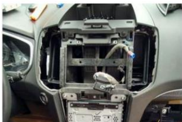
12.Plug the attaching plug of the original car screen,plug the module LVDS wire.
