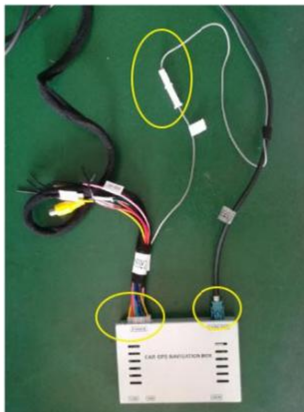
12.Plug the attaching plug of the original car screen,plug the module LVDS wire.
