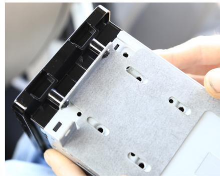
5. Mount mounting frames and facia plate to Double DIN head unit
