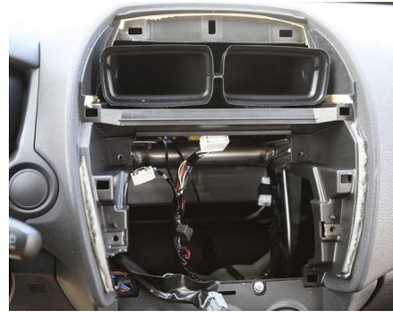
4. Unplug cables carefully Remove OEM head unit
