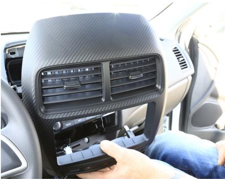
2. Unplug cables and Remove OEM panel
