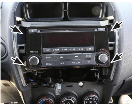
3. Remove 4 screws of OEM head unit
