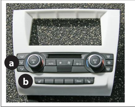
10. Attach air condition control unit (a) and switch bar (b) to replacement fascia plate
