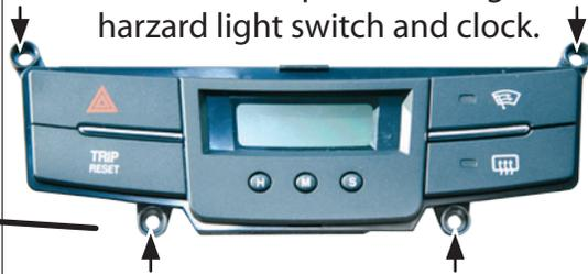
Mount OEM panel to fascia plate **in case of inaccurate mounting position:** cut upper part of OEM panel holder holes (see arrows) to a flat hole in order to get more flexibility for adjustment
