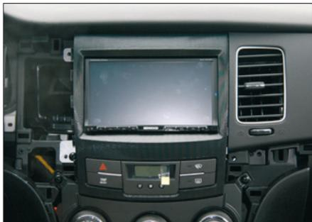
11. Connect harness for panel with hazard light switch
