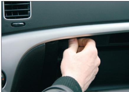
2. Open glove box - remove two screws beneath silver panel
