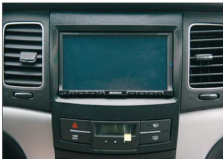
12. Dashboard with installed Double-DIN navigation
