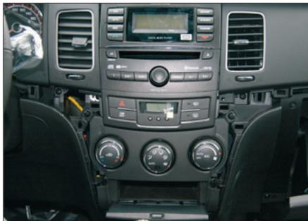
3. Unclip and remove silver panels at left and right side carefully
