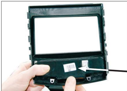
10. Remove OEM panel holding hazard light switch and clock.
