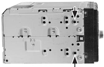
Mount the metal brackets to the double DIN head unit.
