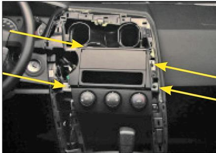
2. Remove the original bracket, which is fixed by four screws at the location of the arrows.
