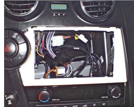
3. Place the new fascia plate on the dashboard and fix it with the four screws.
