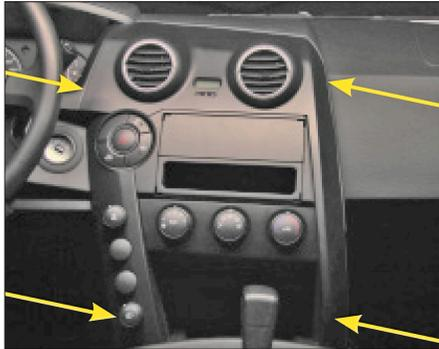
1. Remove the panel under the climate control panel.
