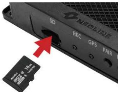
Card removal: carefully press the card and the remove from the slot.
