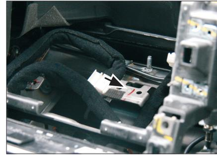
5. Bend down metal in order to clear space for double DIN head unit
