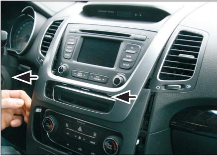
1. Unclip and remove OEM panel
