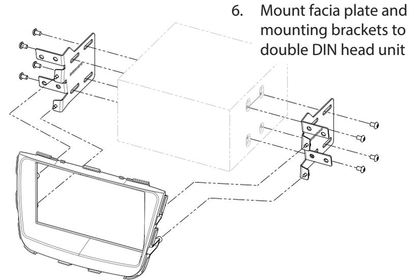
6. Mount fascia plate and mounting brackets to double DIN head unit
