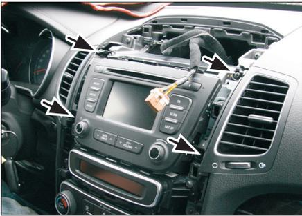
2. Remove screws of air vents
