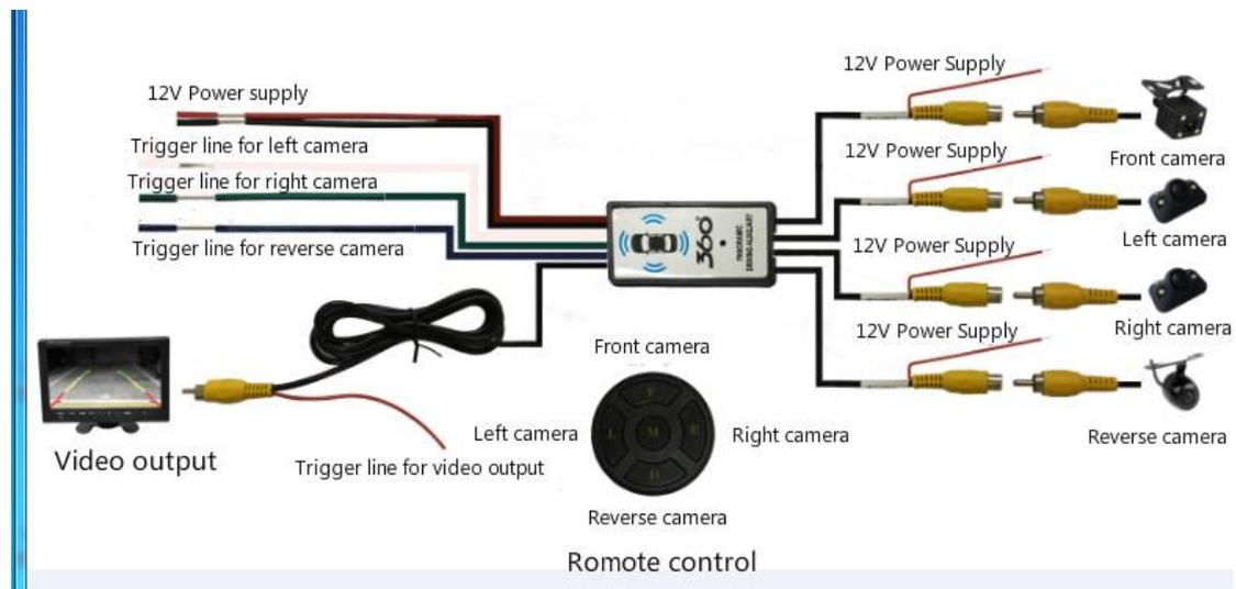
1:Blue trigger line to connect with back-up lamp power
