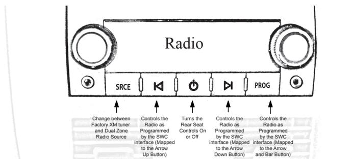
1. Press the power button to turn the RSE Controls on. When Radio is displayed on the RSE Controls, the aftermarket radios rear speaker output will be heard through the headphone jacks. Putting the aftermarket radio into dual zone mode should change the output level of the rear speakers to a fixed level. This allows precise user adjustment from the level knobs on the RSE Controls (refer to aftermarket radio owners manual for model specific dual zone operation).
