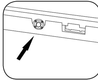
Press the programming button on the side of the interface while OnStar is active to adjust the OnStar volume
