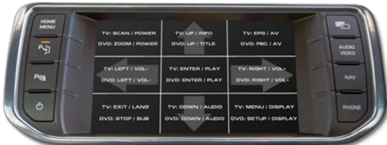
**Note:** Additionally to the control via factory touch-screen, it is possible to install the original IR-sensor of the AV-source. By using the Y-adaptor STA-Y for the IR-Port of the AV-source, the controls of touch-screen AND device's IR-sensor can be connected and used simultaneously. Installation of the IR-sensor is recommended as the controls via touch-screen are limited, and not all functions may be covered.
