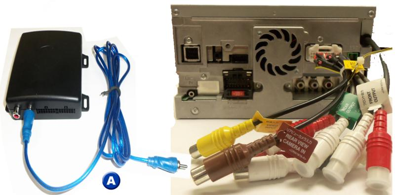
3 Connect the head unit connection lead as shown.
