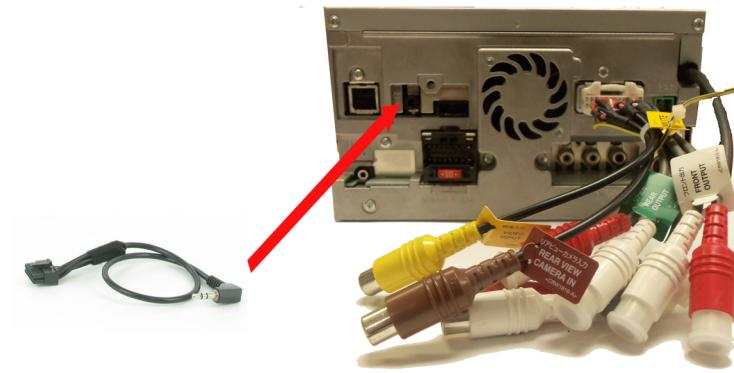
4 Connect the Rear View Camera input to the interface as indicated (*Optional if reverse camera fitted*).
