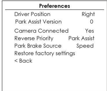
**Reverse Priority\*** - Select which image (Camera or Park Assist) will be shown by default when reversing. The driver can select the desired image by pushing the Mode button (Fig.3) while reversing. (\*Note this option is only available when Camera Connected is set to Yes)
