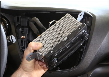
4. Unplug all connectors Remove OEM head unit
