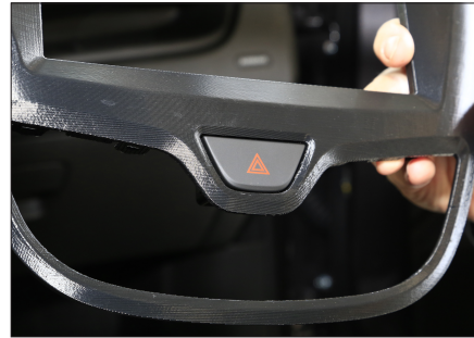
6. Place hazard light switch onto new 2-DIN facia plate
