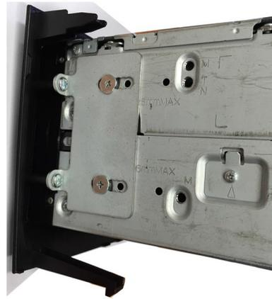
3. Place the aftermarket head unit into the bracket/fascia assembly and line up the mounting holes. Use the screws supplied to secure these together
