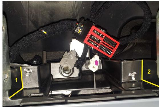
5. Cut the dashboard at the positions shown. Remove the plastic sections 1 and 2. Note the maximum mounting depth is 120mm. For head units over 120mm in depth, the rest of the inner dashboard must be cut
