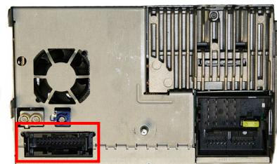
3. Connect the black wire to ground. Connect the red wire with switched plus (+12V).
