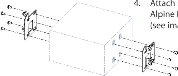
4. Attach mounting brackets to Alpine Double-DIN Navigation (see image below)
