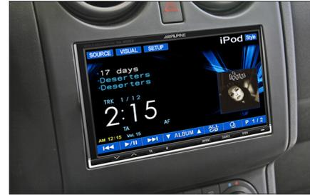
5. Place double DIN navigation, connect all required circuit points. fix it with OEM screws.
