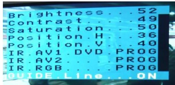
**Note:** If the CAN-box does not support the very vehicle, the guide-lines cannot be used. If supported and activated, the guide-line also show the steering wheel position dependant driving path.
