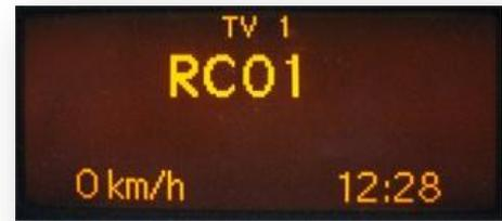
If the vehicle has no MFD display in the instrument panel, you must count the notches when turning the knob (to the right +1, to the left -1). At the same time, remember that the starting point is channel RC01 (the first notch to the right is then already RC02).
