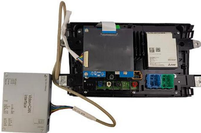
Internal PCB should be inserted inside the monitor, and external PCB board should be fixed on the rear cover of the monitor.
