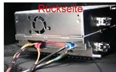
Unplug the insert from the 20-pin socket.
