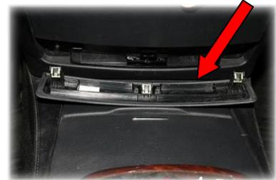
Remove the panel under the drawer (panel is slotted).
