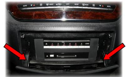
Open the drawer. Loosen the 4 Comand torx screws (2 respectively on each side).
